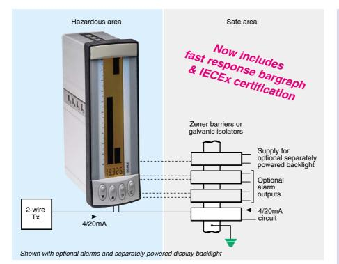
**The BA326C** is an intrinsically safe loop powered indicator that displays the 4/20mA input current on both a 100 segment analogue bargraph and in accurate engineering units on a digital display.
